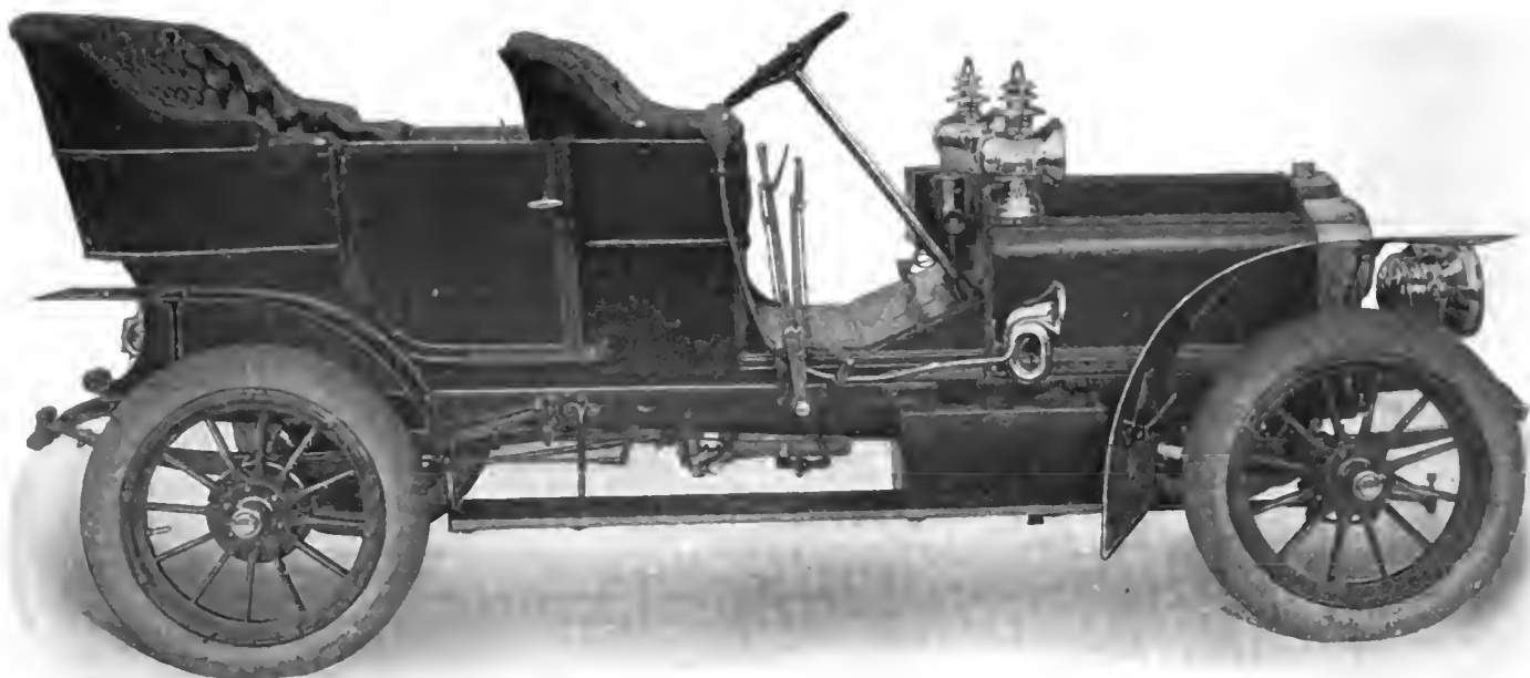
NEW ELMORE 35-HORSEPOWER, FOUR-CYLINDER, TWO-CYCLE MOTOR-IN-FRONT TOURING CAR
